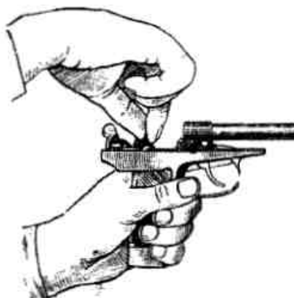
Picture 3.22 Insertion of the slide lock and the sear into the frame
