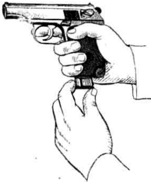
Picture 3.6 Insertion of the Magazine into the Frame
