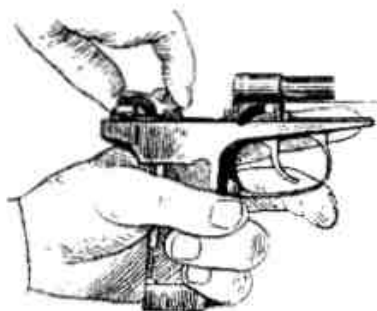
Picture 3.11 Removal of hammer from frame
