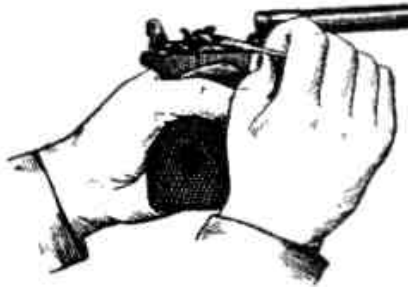
Picture 3.8 Removal of the hammer and slide lock from the frame
