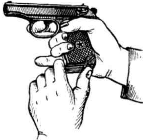
Picture 3.1 Removal of Magazine from the Frame
