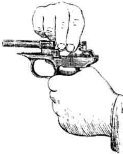
Picture 3.12 Removal of trigger bar with disconnecter from frame
