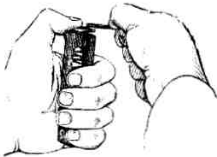
Picture 3.16 Assembly of the magazine
