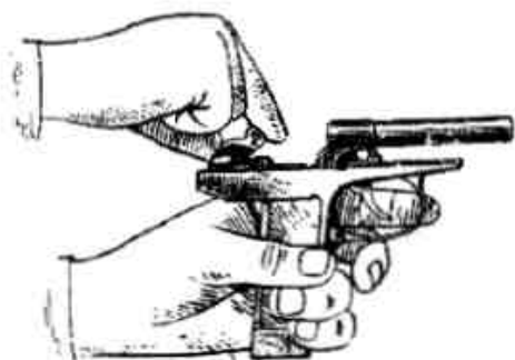
Picture 3.19 Insertion of the hammer into the frame
