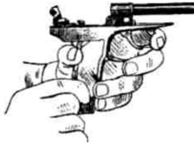
Picture 3.10 Removal of the hammer from the frame
