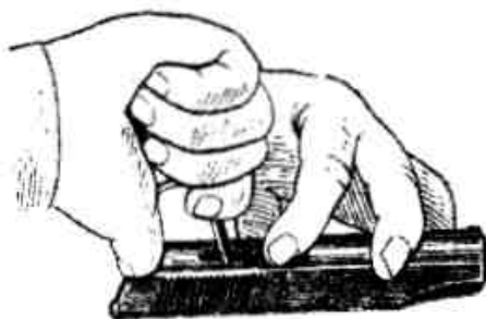
Picture 3.14 Removal of extractor from slide
