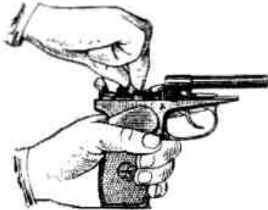
Picture 3.7 Removal of the sear spring hook from the slide lock
