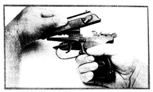
Holding the trigger guard in place with your trigger finger, draw the slide to the rear and lift upward until it comes off the frame.
