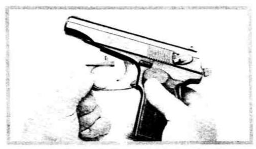
After ensuring that the pistol is unloaded, let the slide go forward. Leaving the hammer cocked, pull down on the front of the trigger guard and push it to the right or left.
